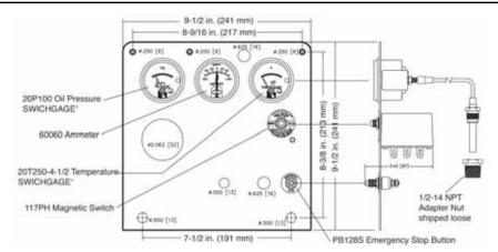
NOTE: This is an standard schematic. if non-standard components are specified, this schematic my not exactly reflect your panel.
